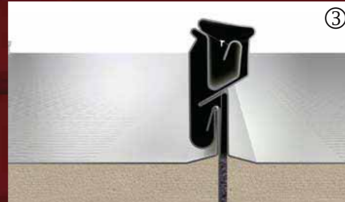
Position the second panel and slide it into place until it is fully attached to the first panel
