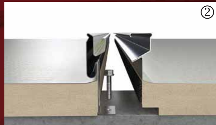
Fasten in place using a fixing bracket, which allows the expansion joints to slide with the possibility of choosing between lateral or upper fastening. For upper fastening, the panel is equipped with a channel to house the bolt.
